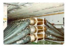
Tyco SL Repeater being deployed as it leaves the ship and before it breaks the water surface
